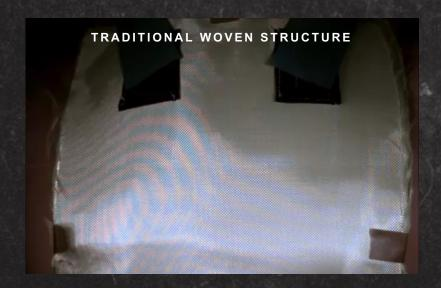
14 plies 600D (24x24) .50psf impacted with 9mm 124gr FMJ @ 955fps
