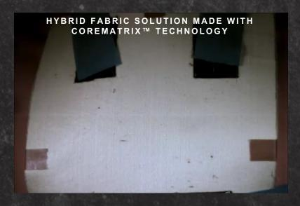
CORE 600D .50psf impacted with 9mm 124gr FMJ @1045 fps
